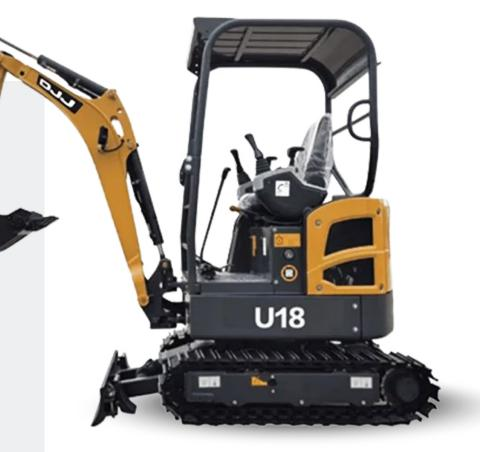
**1880** Operating Weight(kg) **470** Bucket Width(mm) **0.05** Capacity(m<sup>3</sup>)
