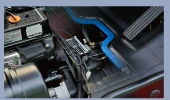
In addition to rubber damper between overhead and frames, compound engine damper and full floating power train achieved flexible connection between frames and driving system, as a result, traveling vibrations and vibrations from the driving system are significantly reduced.
