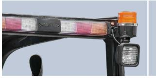
The new efficiency lighting system employs LED illuminant and new type reflector to reduce energy consumption, improve significantly illumination performance and prolong work time.
