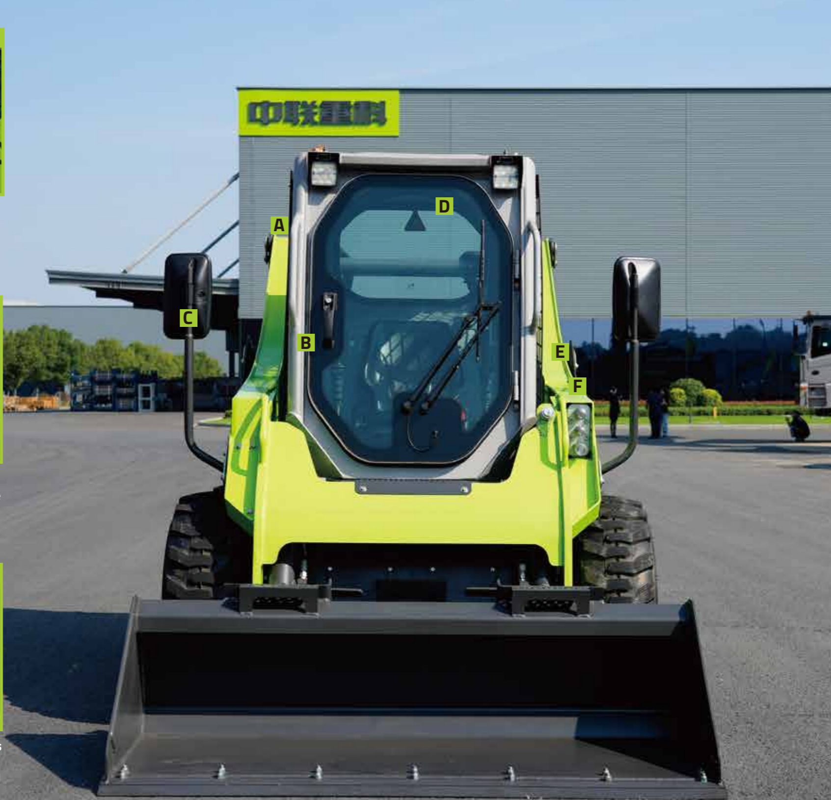
FOPS/ROPS cab A cab certified for FOPS/ROPS provides protection in the event of unforeseen rollovers and falling objects
