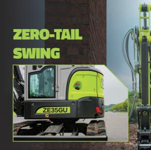
One of ZE35GU's highlights is zero tail swing,its radius of swing will not exceed the width of the track in the full expanded state. This design means that it can work in narrow spaces and on busy roads, not limited by space.
