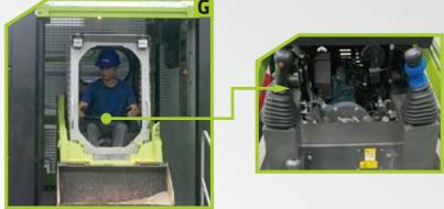
Hydraulic pilot controlling technology making it easy for drivers to control with only 1/3 control power of mechanical control
