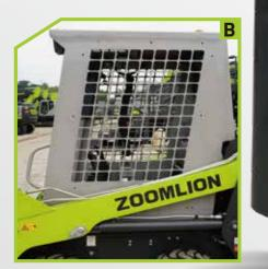
Standard FOPS/ROPS cab with safe certification, ensuring the safety of drivers.
