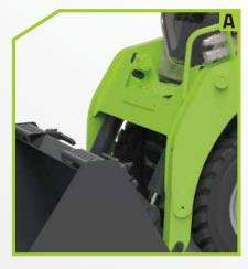
Bucket cylinders and pipelines are equipped with protective cover to prevent from being damaged.
