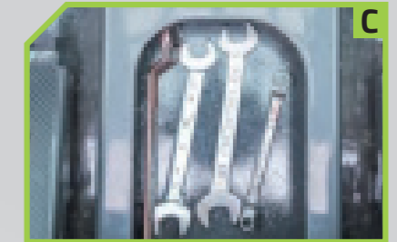
Integrated toolbox The toolbox is integrated into the cab floor for easy storage of tools.
