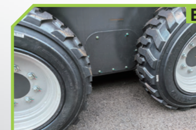
Side-mounted sprocket box Sprocket boxes arranged on the side facilitate daily maintenance and inspection.
