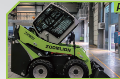
Interior maintenance The cab can be tilted without raising the arm, facilitating access to the hydraulic pump, multi-way valve and pipelines.
