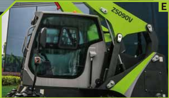
Hydraulic lines are located inside the lifting arm for perfect protection of the hydraulic lines
