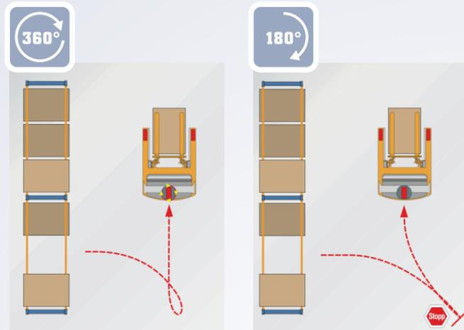
In the mode of 360-degree steering, when steering exceeds 270 degree, the reverse is switched to forward director, no reversing is required, and the truck is switched to advance automatically, no parking is required, with higher efficiency.
