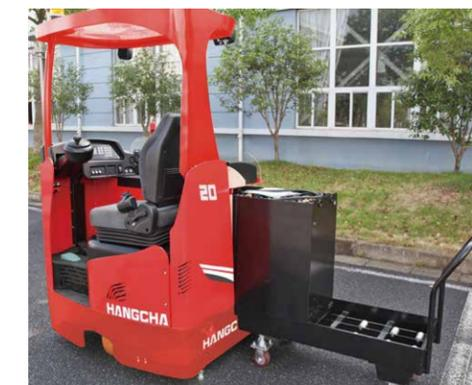
*Standard configuration: Battery side roll-out + trolley(optional)*
