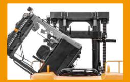
The over-turnable cab and electric tipping cylinder make tipping easier and more labor-saving.
