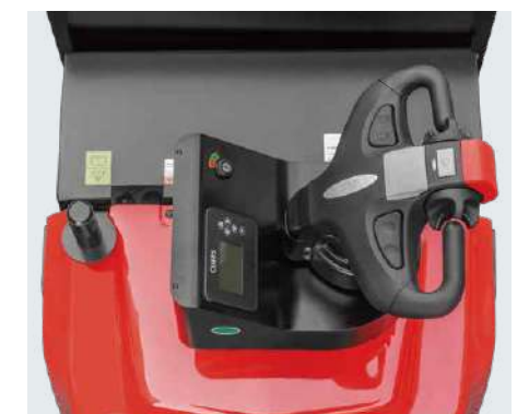
The dashboard with integrated large-screen instruments can be moved sideways to enable the changing battery easier
