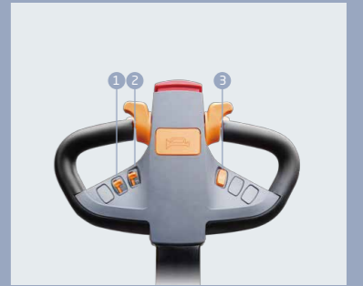
FREI multi-function tiller 1: Forks move forward / backward 2: Forks lifting / lowering 3: Forks tilt forward / backward
