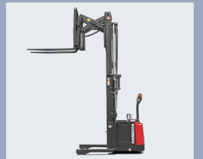
Travel speed is lowered automatically when fork is lifted to specified height
