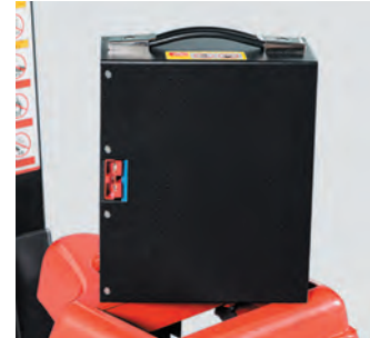
Lithium battery pack
