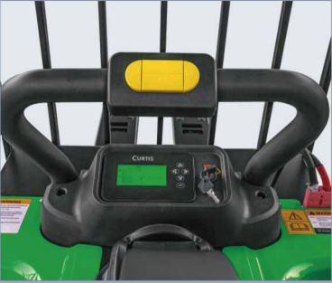
The CURTIS AC Control System
