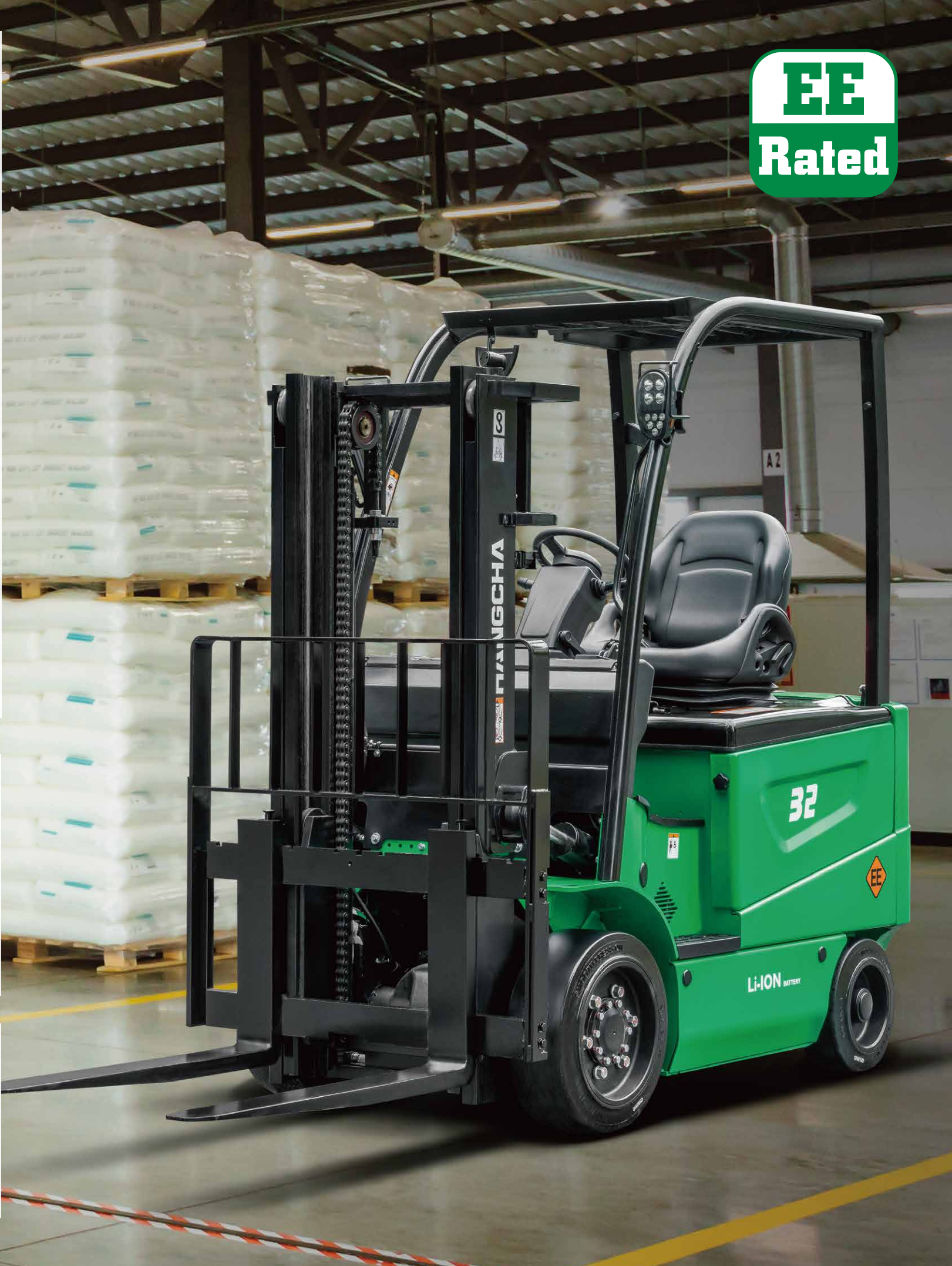
The EE rated forklift's electrical components are enclosed to prevent sparks in hazardous conditions.
