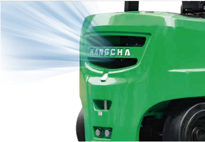
The open counterweight design provides ample airflow for the hydraulic cooling system.
