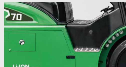
The slip-resistant step and lengthened handrail allow easy in and out of the forklift.
