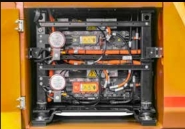
Battery and motor radiator
